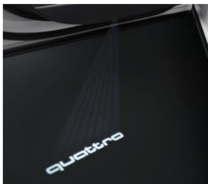
The entry LED projects the quattro lettering onto the ground when the front doors are opened.
