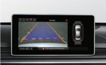
Retrofit solution for reversing camera to aide reversing and parking manoeuvres.
