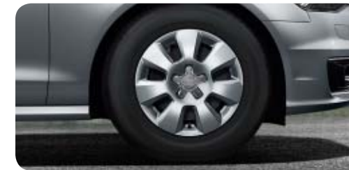
Cast aluminium winter wheels in 7-arm design size 7.5 J x 16 with 225/60 R 16 tyres 1 , can be fitted with snow chains, permissible top speed 210 km/h
