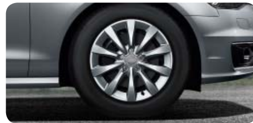
Cast aluminium wheels in 10-spoke design size 8 J x 17 with 225/55 R 17 tyres 1 , optionally with all-season tyres
