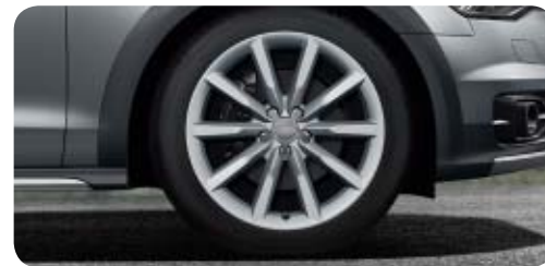
Cast aluminium wheels in 10-spoke design size 8.5 J x 19 with 255/45 R 19 tyres 1 . Only available for A6 allroad quattro
