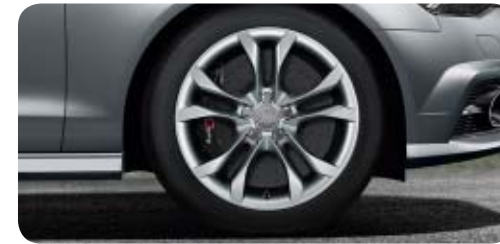
Cast aluminium wheels in 5-parallel-spoke design (S design) size 8.5 J x 19 with 255/40 R 19 tyres 1 . Only available for S6 Saloon and S6 Avant
