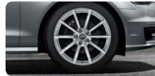
Audi Sport cast aluminium wheels in 10-spoke design 2 size 8.5 J x 19 with 255/40 R 19 tyres 1 (on A6 allroad quattro with 255/45 R 19 tyres 1 )
