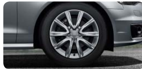
Cast aluminium wheels in 5-V-spoke design size 8 J x 18 with 245/45 R 18 tyres 1
